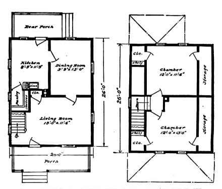
Fig. 49.—PICTURE AND PLANS OF TYPICAL 5-ROOM HOUSE WITH WATER AND ELECTRIC LIGHT.
